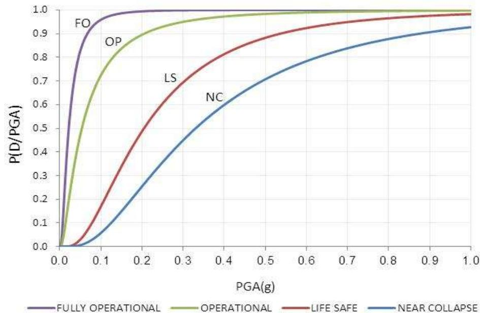
Figure 7: Overall fragility curves for all structures
